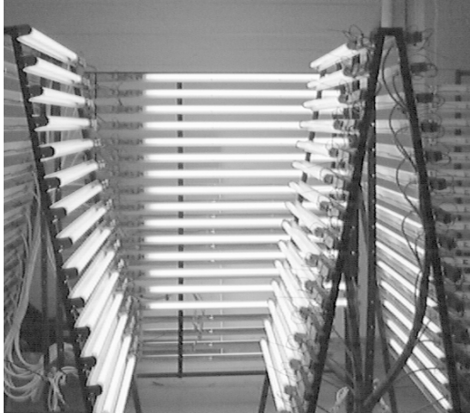
Fig. 6 Lamp life test. Lamps were burned in open test racks.
