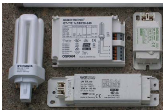
Figure 7 TC-D lamp 18 W, energy efficient magnetic ballast and electronic ballast for this (top) and B1 magnetic ballast for a common-place T8 lamp of equal power rating (bottom)
