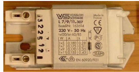
Figure 2 Equivalent ballast as in Figure 1 – later model and different manufacturer. Power factor ( \lambda ) ratings are significantly higher for higher lamp power ratings!
