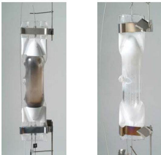
Conventional magnetic or electronic ballast Metrolight electronic ballast with High Frequency MicroStart™ Ignition
