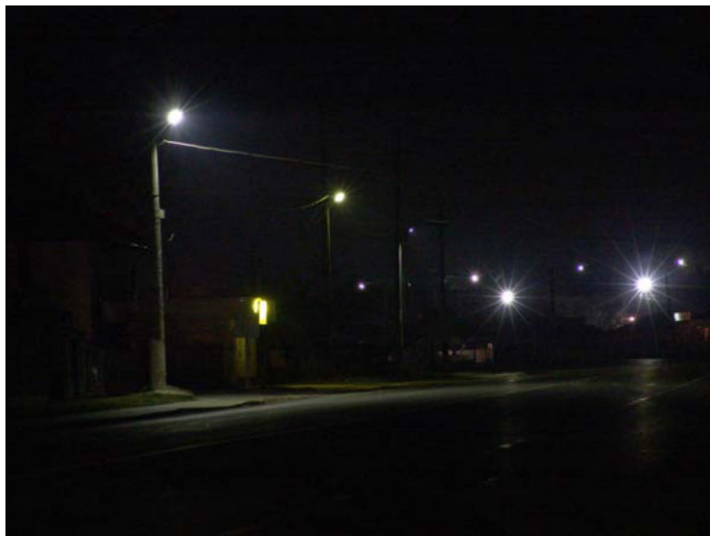
Figure 5 The local effect of the luminaire and the glare
