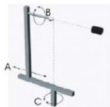
Figure 1 Mechanical Movements of Goniophotometer (17)
